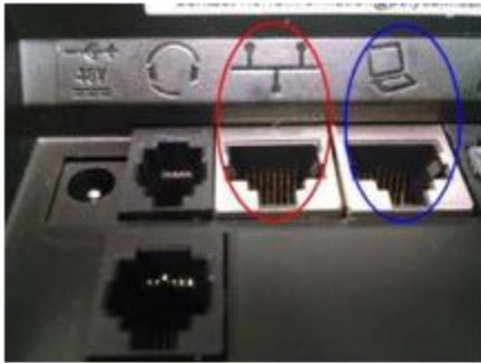
Passthrough ethernet connection to PC (optional; extra cable not included)
